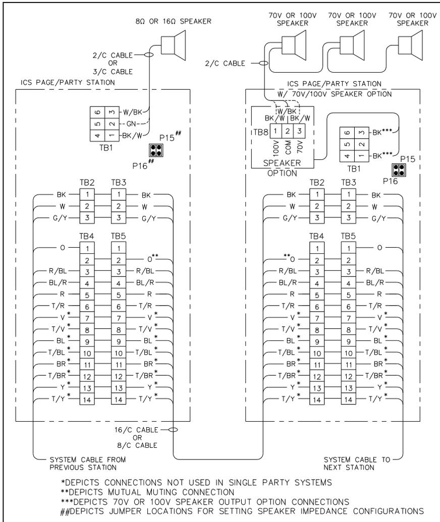
Figure 3. Typical installation wiring configuration
